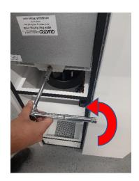
4. An acorn-nut on the back of the bolt will stop the mechanism once it is fully "removed". Slide out the HEPA filter once the track comes out, demonstrated below.
