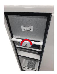
Tighten the HEPA seal mechanism – clockwise rotation – until gasket is fully compressed.
