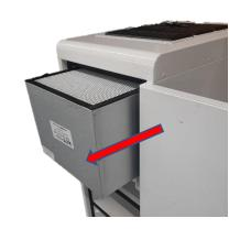
5. Insert new HEPA filter onto the filter track – gasket facing upwards
