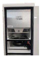
Use socket wrench - counter-clockwise rotation - on the bolt centered on the HEPA seal mechanism.
