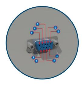
Pin 1 Dry Contact Board Return/Board Ground
